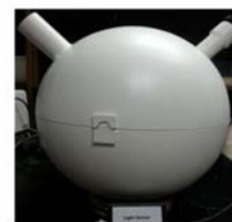
An integrating sphere for the undergraduate lab with sensor
